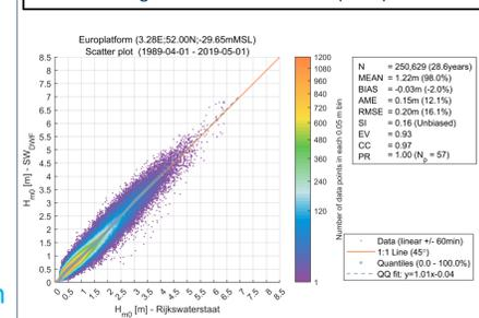
Significant wave height validation at Europlatform (1989-2016)
