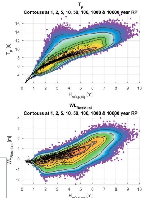
Scatter plots show Tp (top) and residual water level (bottom) against Hm0, based on **1e+6** years of simulation
