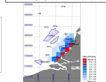
Difference of mean wind speed at 10m between original and corrected CFSR (2017)
